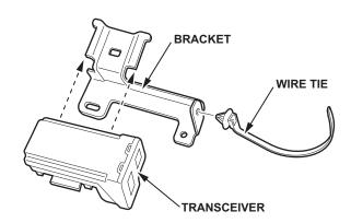
13. Connect the wire tire with clip to the bracket.
