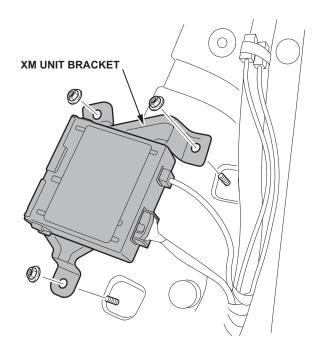
12. Slide the transceiver onto the bracket.
