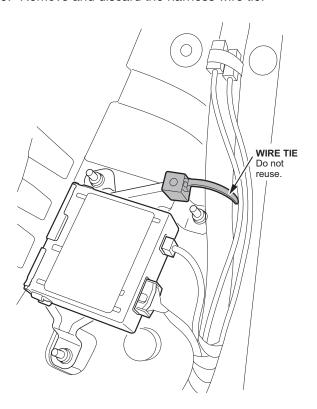
11. Remove the three XM unit bracket nuts.
