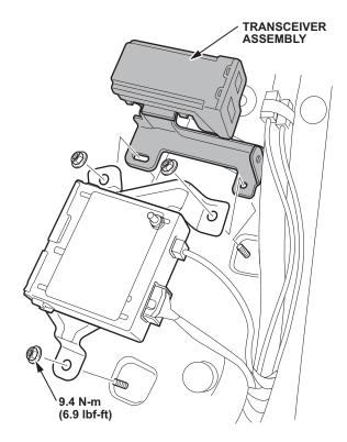
15. Reinstall the XM unit using the three nuts and torque to 9.4 N•m (6.9 lbf-ft).
