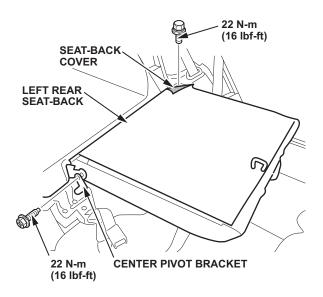
5. Remove the center pivot bracket and remove the left rear seat-back.
