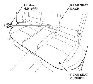
7. While pushing down on the seat cushion, pull the seat hook handles to release the hooks.
