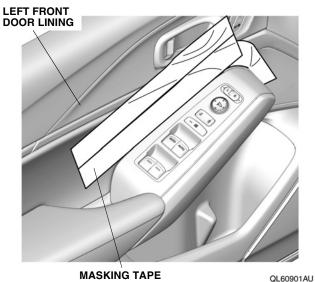
3. Remove the left front door switch panel.
