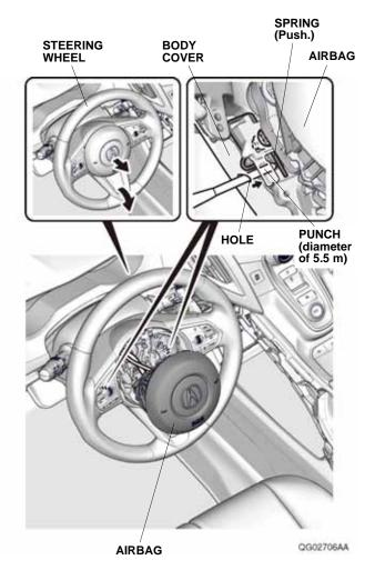
8. Insert a punch (diameter of 5.5 mm) through the left hole of the body cover, and push the spring to release the airbag. Repeat for the other side.
