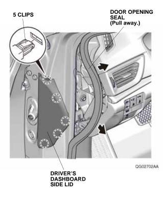
4. Remove the driver's dashboard side vent.
