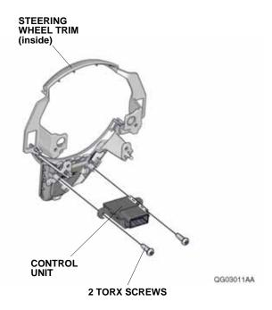
34. Plug the new cable reel cord 14-pin connector into the control unit, and install the steering wheel trim to the new steering wheel with five self-tapping screws removed in step 28.
