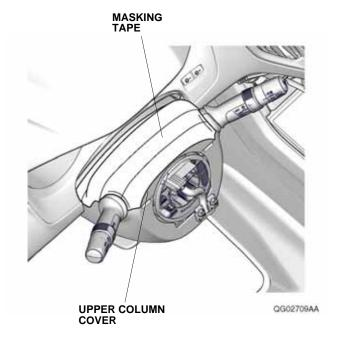
15. Using a plastic trim tool, release the upper column cover and secure it to the dashboard with masking tape.
