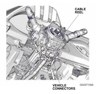
19. To prevent turning from the cable reel, apply masking tape to it. Remove the cable reel.
