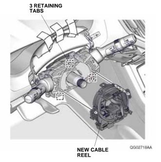
24. Plug the vehicle connectors into the new cable reel.
