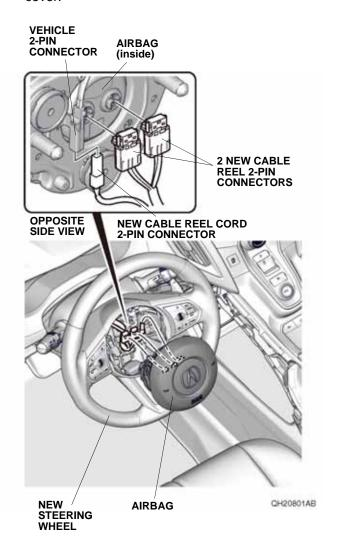
44. Install the airbag to the new steering wheel.
