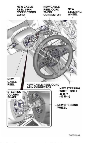
42. Install the new steering wheel bolt. Torque it to 36 lb-ft (49 N·m).
