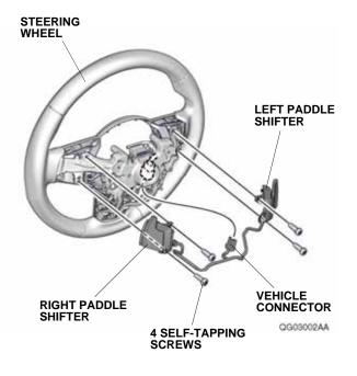
27. Remove the two vehicle switches, and unplug the vehicle connectors.
