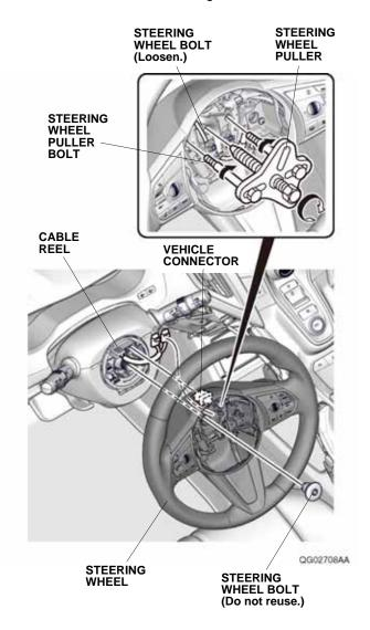
12. Using a steering wheel puller, release the steering wheel.
