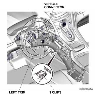
6. Remove the driver's dashboard lower cover, and unplug the vehicle connectors and vehicle sensor.
