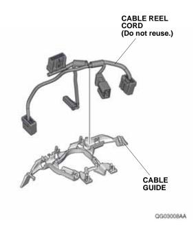
31. Install the new cable reel cord to the cable guide.
