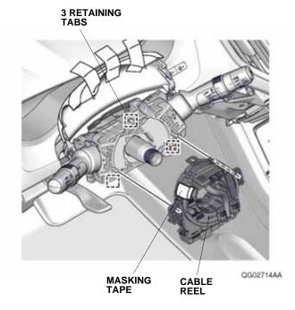
20. Remove the masking tape. Remove the steering angle sensor.
