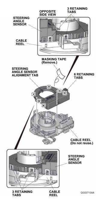
21. Install the steering angle sensor to the new cable reel
