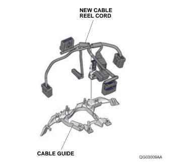
32. Plug the new cable reel cord 4-pin connector into the new steering wheel 4-pin connector, and install the cable guide to the new steering wheel.
