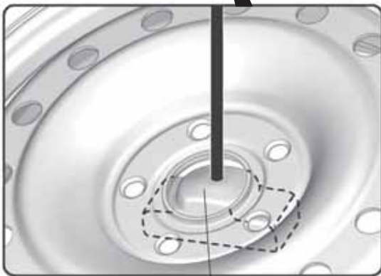
Bracket position is incorrect.
