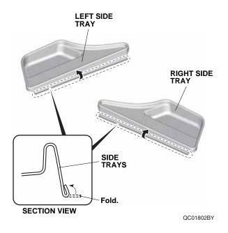
5. Place the left and right side trays in the trunk. Insert the folded ends of the side trays into the gap as shown.
