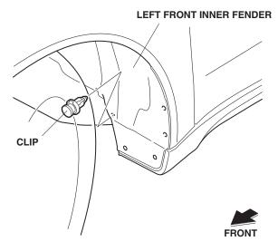
4. Install the left front splash guard to the left front inner fender with two self-tapping screws and the clip removed in step 3.
