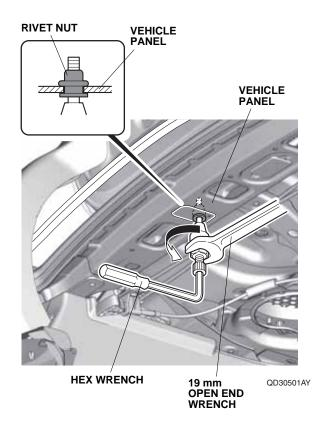
6. Remove the rivet nut tool from the rivet nut by turning the hex wrench counterclockwise.
