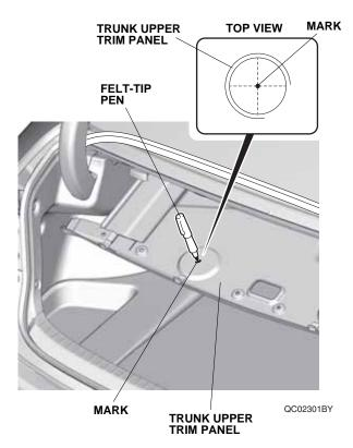
8. Using a pushpin, pierce the trunk upper trim panel at the mark made in step 7.
