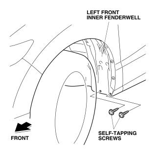
4. Install the left front splash guard to the left front inner fender with two washer-screws and the two self-tapping screws removed in step 3. Tighten in the order  $1 \rightarrow 2 \rightarrow 3 \rightarrow 4$ .
