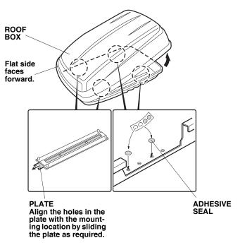
3. Attach an adhesive seal over each of the four unused mounting holes (two on each side) at the rear of the base of the box. The seals will help prevent water from entering the roof box. Then, remove the roof box from the crossbars. 4. Using isopropyl alcohol on a shop towel, clean four brackets B where the small pads will attach. Remove the adhesive backings from the small pads, and attach them to the brackets B.
