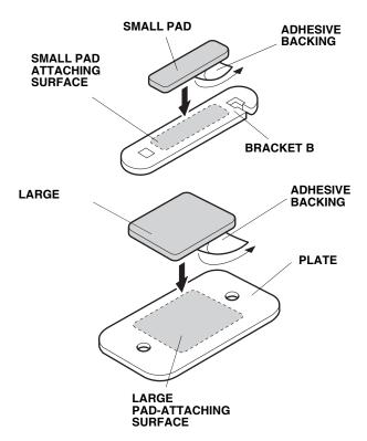
5. Using isopropyl alcohol on a shop towel, clean the four plates where the large pads will attach. Remove the adhesive backings from the large pads, and attach them to the plates.
