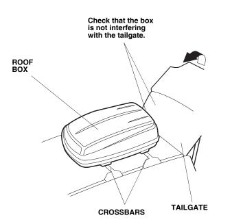
Open the roof box, and align the holes in the plate with the mounting location at the forward crossbar. The plate is located at the front of the base of the roof box.
