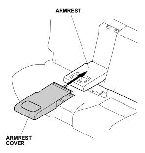
5. Raise the armrest. Pull the armrest cover between the armrest and left rear seat back, and secure the fasteners on the armrest cover as shown.
