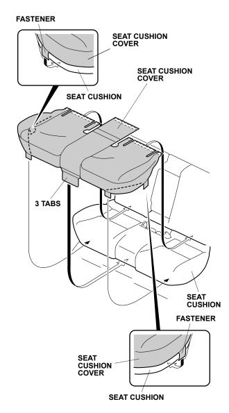
Put the seat cushion cover around the center seat belt buckles as shown. Insert the seat cushion cover between the rear seat back and the rear seat cushion, and secure the fasteners to the rear seat cushion.
