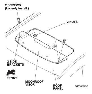
16. Position the moonroof visor with equal spacing on each side. Check that the rubber molding is not twisted or rolled under the visor.
