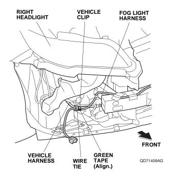
40. With the help of an assistant, bring the front bumper close to the vehicle, and plug the two fog light harness 2-pin connectors or two vehicle 2-pin connectors to the two LED fog lights.
