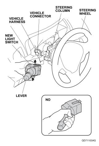
14. Plug the vehicle connector to the new light switch.
