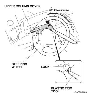
3. Turn the steering wheel 180° counterclockwise. Using a plastic trim tool, release the lock as shown.
