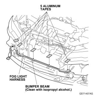
38. Secure the fog light harness to the bumper beam with two wire ties.
