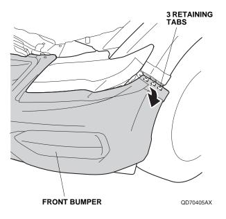
Release the six retaining tabs on each side.
