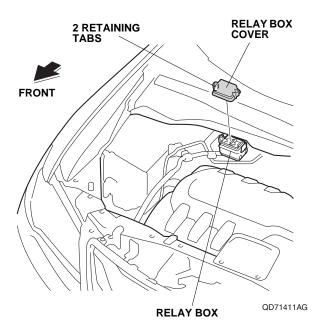
43. Install the relay into the relay box.
