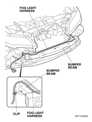
37. Using isopropyl alcohol on a shop towel, thoroughly clean the areas where the aluminum tapes will attach. Secure the fog light harness to the bumper beam with five aluminum tapes.
