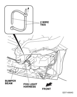
39. Align the green tape on the fog light harness with the vehicle clip, and secure the fog light harness to the vehicle harness with one wire tie.
