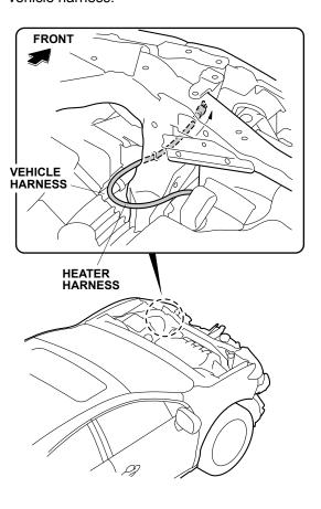
22. Route the heater harness under the left headlight, and secure it to the side duct with one black wire tie (point C).
