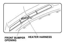
30. Install the protective cap to the front bumper as shown.
