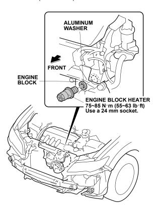
18. Plug the heater harness connector into the engine block heater.
