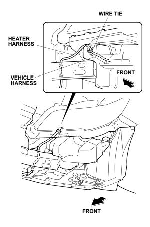
27. Secure the heater harness to the vehicle harness with one black wire tie.
