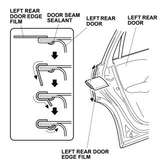
23. Using a shop towel, wipe the excess 3M protective tape application solution from the left rear door edge film. Allow the left rear door edge film to dry thoroughly.
