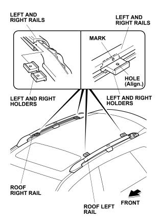
4. Align the hole in each holder with the mark on the inside of the roof rail.
