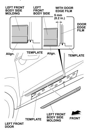
7. While applying light pressure against the left front body side molding, carefully remove the taped adhesive backings.
