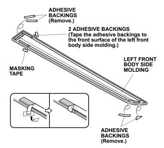
Align the left front body side molding with the template and attach it to the left front door as shown. NOTE: If the vehicle is equipped with door edge film, attach the left front body side molding at the indicated position.
