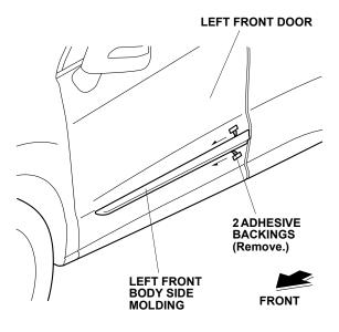
8. Using a rubber roller, apply pressure against the left front body side molding and roll from one end to the other.
