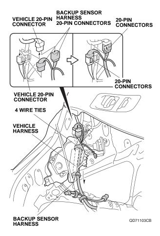
23. Secure the backup sensor harness to the vehicle harness with four wire ties.
