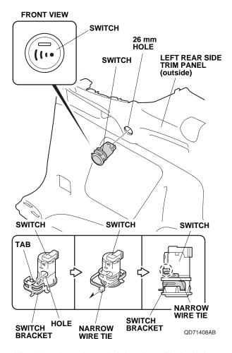
41. Align the tab on the switch bracket with the hole on the switch and secure the switch bracket to the switch with one narrow wire tie.
