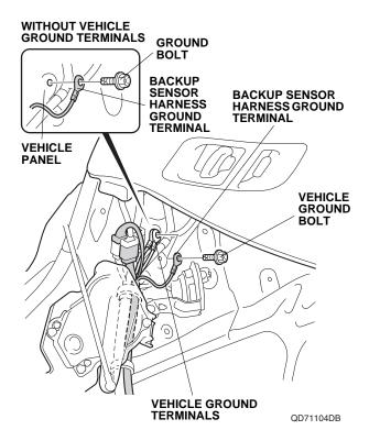
25. Secure the backup sensor harness ground terminal to the vehicle ground terminals with the vehicle ground bolt just removed. Do not put the ground terminal calkings on top of one another.
