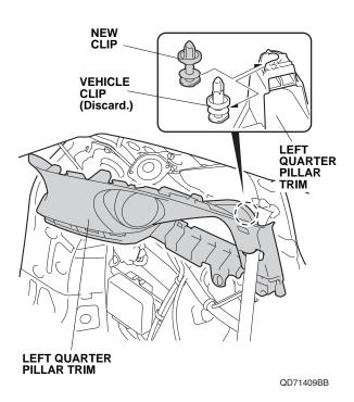
43. Check the overlap between the headliner and the quarter pillar trim, and install the new clip to the left quarter pillar trim.
