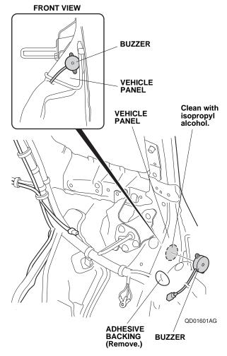
27. Remove the adhesive backing from the buzzer and attach the buzzer to the vehicle panel in the location shown.
