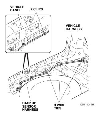
37. Secure the backup sensor harness to the vehicle panel with two clips on the backup sensor harness.
