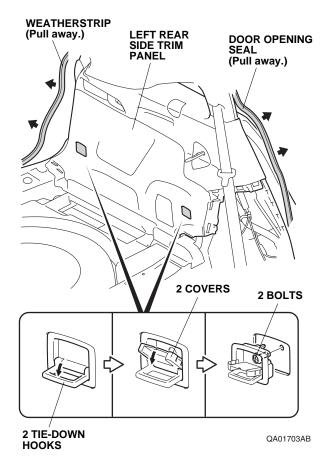
10. Using an impact screwdriver, remove the two tiedown hooks.
