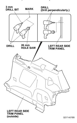
40. Install the switch into the 26 mm hole in the left rear side trim panel.
