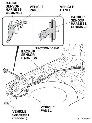
35. Route the backup sensor harness through the hole, and seat the grommet on the backup sensor harness in the vehicle panel hole.
