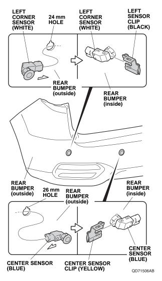
52. Secure the left corner sensor (white) and center sensor (blue) with left sensor clip (black) and center sensor clip (yellow) as shown.
