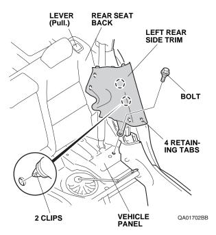
8. Pull the lever, and fold down the rear seat back.
