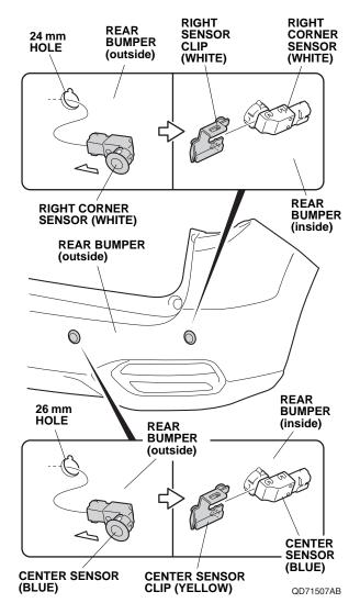
54. Secure the right corner sensor (white) and center sensor (blue) with right sensor clip (white) and center sensor clip (yellow) as shown.
