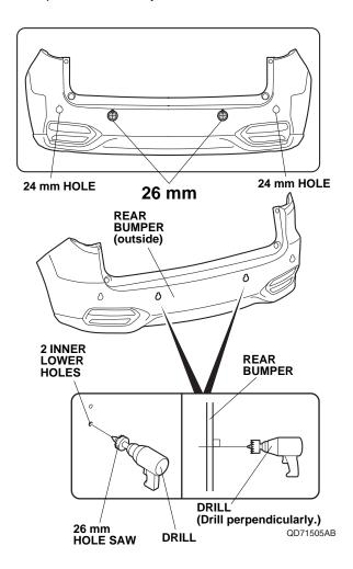
51. Install the left corner sensor (white) and center sensor (blue) to the rear bumper.
