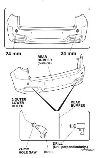
50. While wearing eye protection and drilling from painted side of the rear bumper, enlarge the two lower 3 mm inner holes to 26 mm using a 26 mm hole saw.
