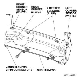
56. Secure the two subharness clips to the two center sensor clips as shown.
