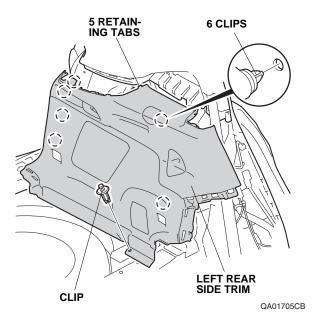
14. Release the wire and remove the lever, then remove the left rear side trim panel.
