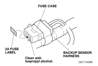
22. Unplug the vehicle harness 20-pin connector, and plug it into the backup sensor harness 20-pin connector. Plug the remaining backup sensor harness 20-pin connector into the vehicle 20-pin connector.
