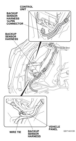
33. Secure the backup sensor harness to the vehicle panel and vehicle harness with one wire tie.
