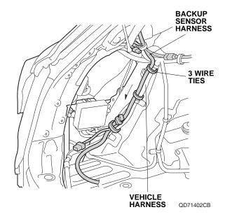
32. Plug the backup sensor harness 14-pin connector into the control unit.
