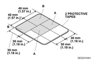
27. Using isopropyl alcohol on a shop towel, thoroughly clean the vehicle panel where the protective tape will attach. Attach one piece of protective tape A to the vehicle panel as shown.
