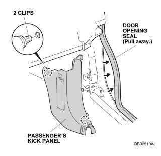
6. Remove the passenger's front side outer trim.
