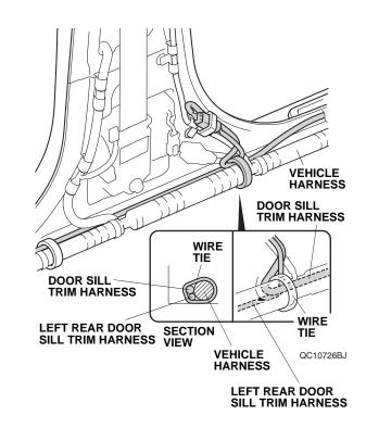
49. Secure the door sill trim harness to the vehicle harness with two wire ties.
