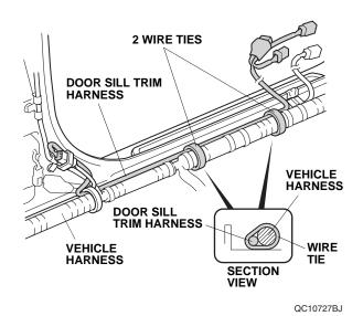
50. Plug the door sill trim harness 2-pin connector into the left front door sill trim 2-pin connector.
