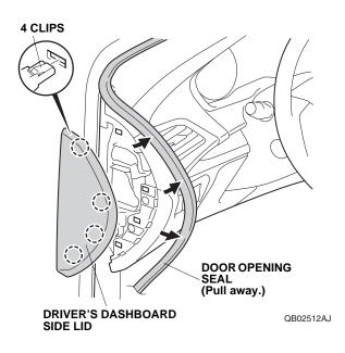
8. Remove the driver's dashboard side vent.
