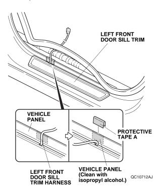
28. Install the protective clip to protective tape A on the vehicle panel.
