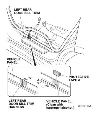
39. Install the protective clip to protective tape A on the vehicle panel.
