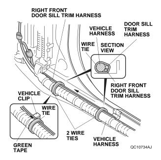
60. Line up the green tape on the door sill trim harness with the vehicle clip and secure the right front door sill trim harness and door sill trim harness to the vehicle harness with two wire ties.
