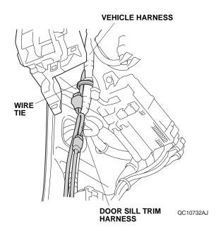
58. Bundle up the excess door sill trim harness and secure it and the 2-pin connectors to the vehicle harness with one wire tie.
