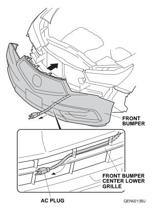
22. Secure the heater harness to the front bumper center lower grille with two black wire ties.
