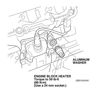
12. Plug the heater harness connector into the engine block heater.
