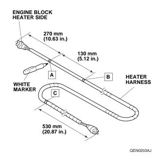
9. Install the one wire tie with clip to the heater harness at point A as shown.
