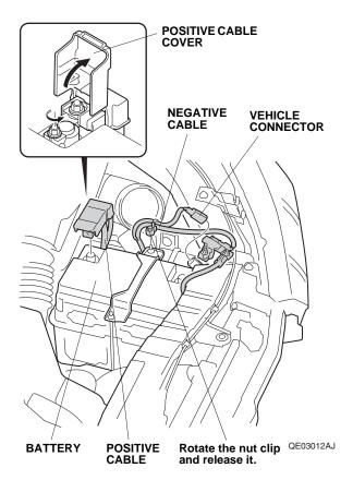
5. Remove the battery, battery holder, battery cover, and the battery tray.
