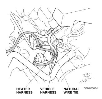
15. Route the heater harness toward the fan shroud and secure the heater harness to the fan shroud rib with the one natural wire tie at the point B.
