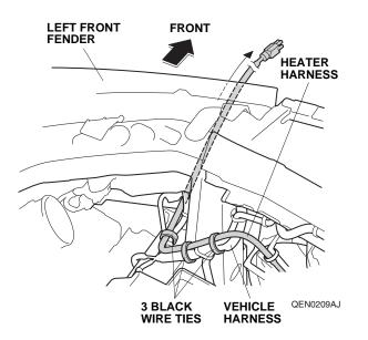
18. Route the heater harness down under the front bumper beam and secure the heater harness to the left front air guide plate hole with one black wire tie at point [C].
