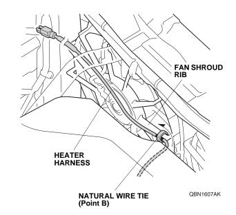
16. Route the heater harness across the fan shroud and secure the heater harness to the fan shroud ribs with three natural wire ties and one black wire tie.
