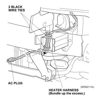
20. Connect two black wire ties together and secure the heater harness to the left front bumper beam extension with the connected black wire ties.
