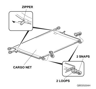
• Attach four loops from the cargo net to the two anchors. Attach two snaps from the cargo net to two cargo hooks.
