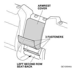
6. Secure the fastener to the bottom of the left second row seat-back.
