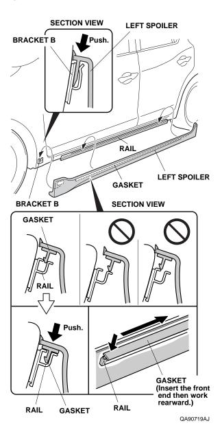
27. Lightly tap the left spoiler to remove any gap between the left spoiler and the left rear fenderwell.
