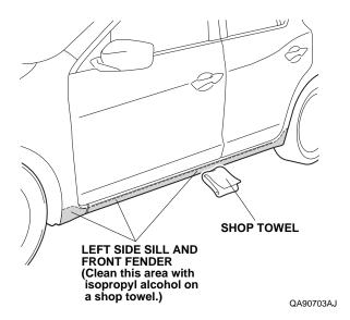
9. Line up template B with the two clips, and attach it to the left front fender with masking tape.
