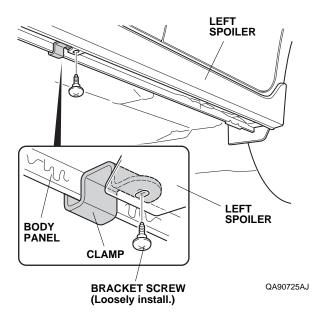
36. Assemble the screw and the washer-nut.
