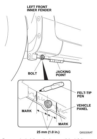
2. Remove the bolt from the bottom of the left front fender.
