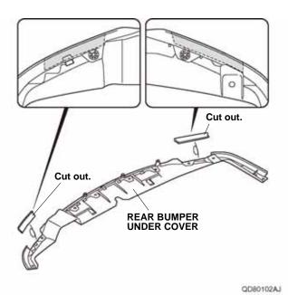
5. Line up the templates No. 1 and No. 2 with the rear bumper as shown. Attach the templates to the rear bumper using masking tape.
