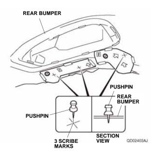
7. Turn the template No. 2 over, and line up the templates No. 2 and No. 3 with the rear bumper as shown. Attach the templates to the rear bumper using masking tape.
