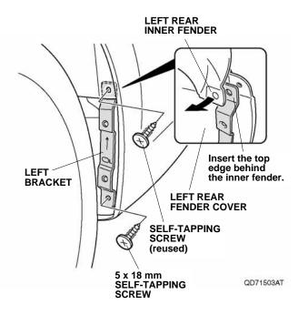
4. Install the 5 x 18 mm self-tapping screw.
