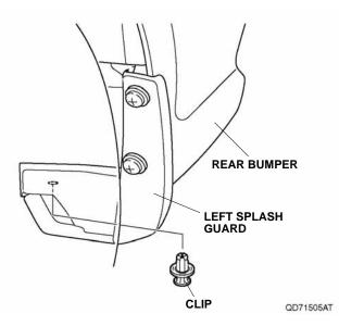
7. Repeat steps 1 through 6 to install the right splash guard on the right side of the vehicle.
