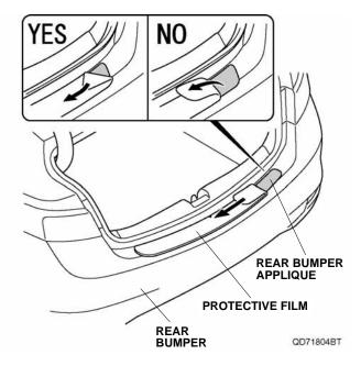
11. Repeat step 8 for the center of the rear bumper applique lower section.
