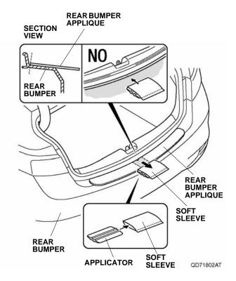
8. Starting from the center and working rearward, use the soft sleeve to smooth out the center of the upper section on the rear bumper applique.
