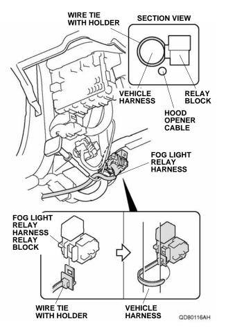
40. Unclip the vehicle connectors from the vehicle panel.
