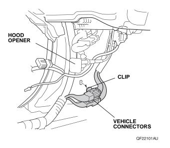
41. Remove the vehicle connector from the vehicle 18-pin connector.
