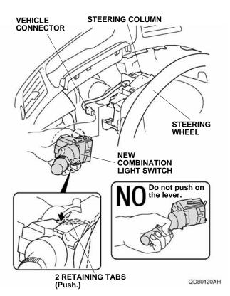
53. Plug the vehicle connector to the new combination light switch. Make sure the vehicle harness has some slack.
