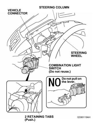
51. While pushing the two retaining tabs, slide the combination light switch out and remove it from the steering column.
