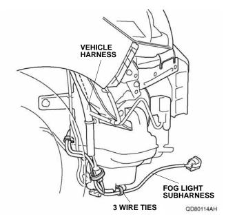
34. Line up the green tape on the fog light subharness with the vehicle clip as shown, and secure the fog light subharness to the vehicle harness with one wire tie.
