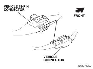
42. Remove the clip from the vehicle 18-pin connector, and install the supplied clip on the vehicle 18-pin connector.
