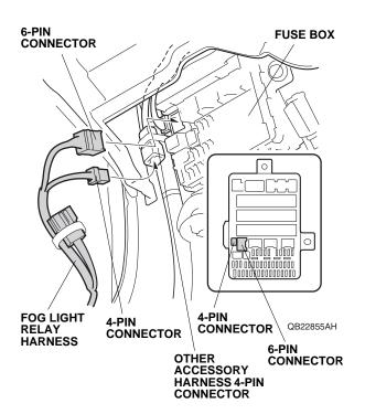
49. Secure the fog light relay harness to the vehicle harness with three wire ties.
