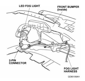
23. Secure the six clips on the fog light harness to the six ribs on the front bumper as shown.
