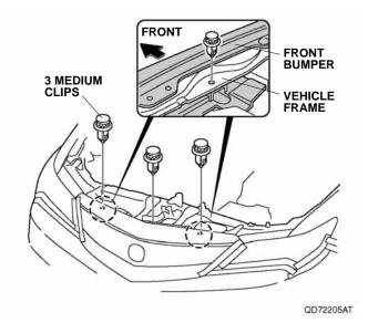
• Remove two self-tapping screws, two bolts, two short clips, and 12 medium clips.
