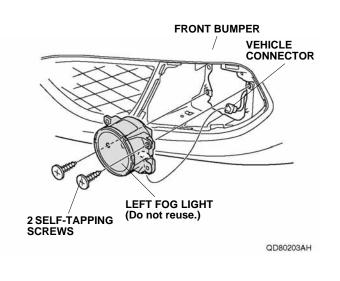
62. Plug the vehicle connector into the LED fog light. Install the LED fog light to the front bumper with three self-tapping screws.
