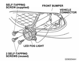
Install the left fog light cover to the front bumper and 63. tighten one self-tapping screw.
