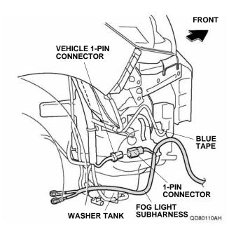
28. Plug the vehicle 1-pin connector into the fog light subharness 1-pin connector.
