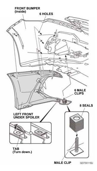
21. Loosely install one clip holder onto each male clip on the left front under spoiler. Do not tighten the clip holders at this time.
