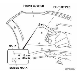
14. Using a pushpin, pierce the center of the mark made in step 13 on the front bumper.
