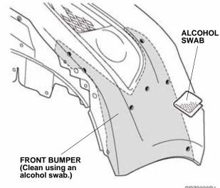
19. Peel back about 20 to 40 mm (0.8 to 1.6 in.) of adhesive backing from each adhesive strip, and tape the ends to the front surface of the left front under spoiler.
