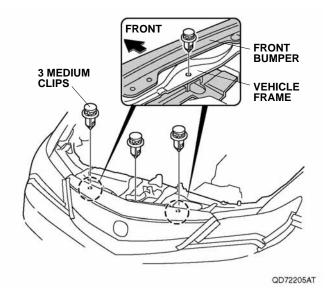
Remove 2 self-tapping screws, 2 bolts, 2 short clips, and 12 medium clips.
