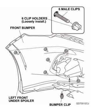
22. Secure the left front under spoiler to the front bumper with one bumper clip.
