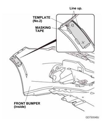
11. Using a pushpin, pierce the center of one mark on the template.
