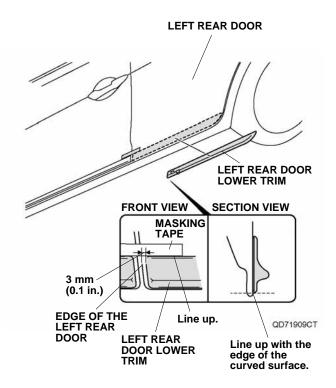
12. While applying light pressure to the rear door lower trim, carefully remove the two adhesive backings. Using the palm of your hand, firmly press the left rear door lower trim onto the left rear door.
