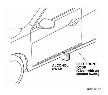
2. Peel back the ends of two adhesive backings on the left front door lower trim and attach them to the front of the trim with masking tape.
