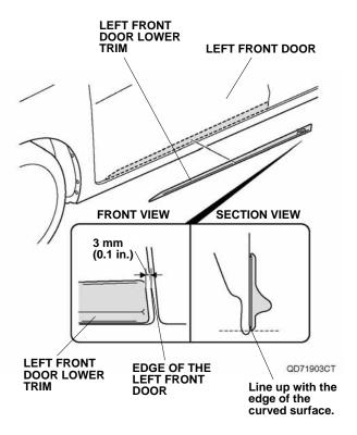
While applying light pressure to the front door lower trim, carefully remove the two adhesive backings.
