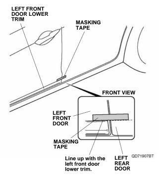
9. Peel back the ends of two adhesive backings on the left rear door lower trim and attach them to the front of the trim with masking tape.
