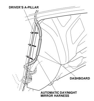
21. Line up the green tape on the automatic day/night mirror harness with the vehicle clip, and secure the automatic day/night mirror harness to the vehicle harness with one wire tie as shown.
