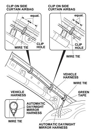
22. Secure the automatic day/night mirror harness to the vehicle harness with three wire ties as shown.
