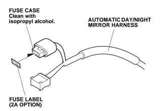
15. Attach the fuse label to the automatic day/night mirror harness fuse case.
