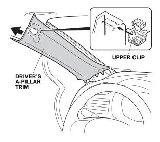
8. Remove the remaining upper clip from the driver's A-pillar.
