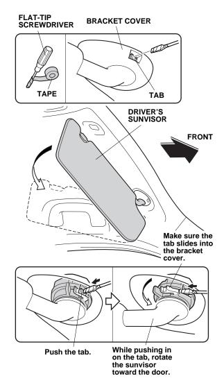
• Unplug the vehicle connector, and remove the driver's sunvisor.
