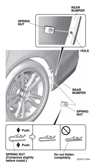
4. Get the left bracket and install two spring nuts on it in the direction shown.
