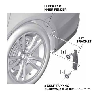
Secure the left bracket to the rear bumper using a 6. 5 x 25 mm self-tapping screw. Thread the screw into the spring nut through the left rear inner fender.
