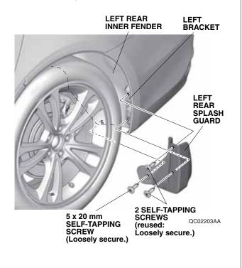
10. Loosely secure the left rear splash guard to the rear bumper with one additional 5 x 20 mm self-tapping screw.
