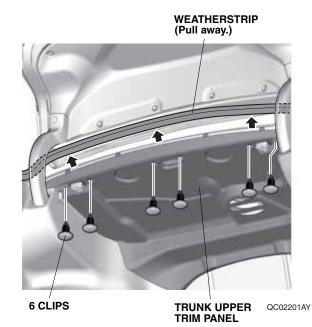
2. Pull down the trunk upper trim panel. Push the tab, then pull down the right seat-back release lever to release the hook and remove the lever. Remove the left seat-back release lever the same way.
