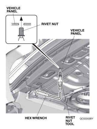
5. While holding the rivet nut tool with the hex wrench, use a the 19 mm open end wrench to rotate the tool counterclockwise.
