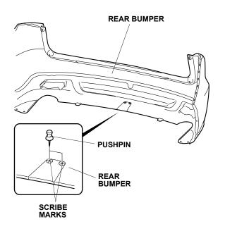
5. While wearing eye protection, drill the two pierced marks with a 3 mm drill bit, then enlarge the holes with a 20 mm hole saw.
