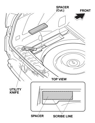
9. Using a utility knife, cut out an additional piece of the left spacer at the measurements shown.
