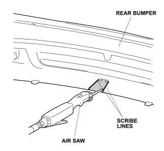
7. Using the air saw, cut the rear bumper between the two 20 mm holes. Remove any burrs.
