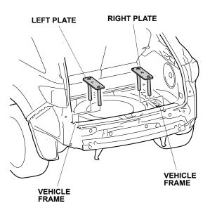
With the help of an assistant, insert two spacers between the trailer hitch and the vehicle frame. Mount the trailer hitch using two loosely-installed 12 x 40 mm bolts with spring washers and plain washers. Be careful that the spacers do not fall out during installation.
