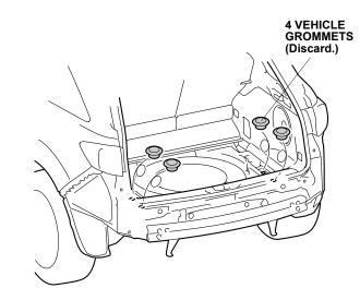
12. Insert the right and left trailer hitch plates through the grommet holes.
