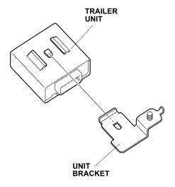
13. Secure the trailer unit to the vehicle panel with a flange nut as shown.
