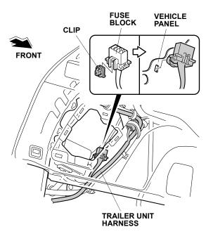
22. Secure the fuse block on the trailer unit harness to the vehicle panel. Go to step 24.
