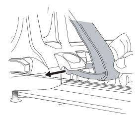
7. Rotate the buckle up to lock it into the base. Repeat this step for the remaining bases.
