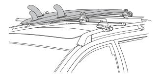
5. Adjust the position of the bases so that the bottom of the surfboard rests on the rubber part of the bases. Tighten all knobs firmly and evenly.
