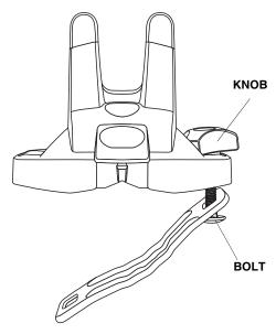
2. Position the base on the crossbar. Loosely install one bolt and knob as shown.
