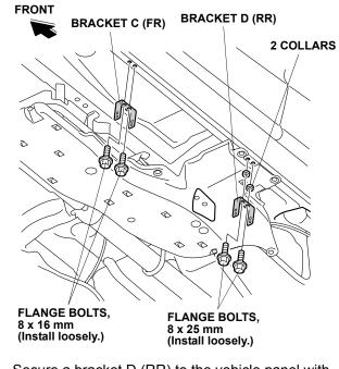
16. Secure a bracket D (RR) to the vehicle panel with two collars and two loosely-installed 8 x 25 mm flange bolts.
