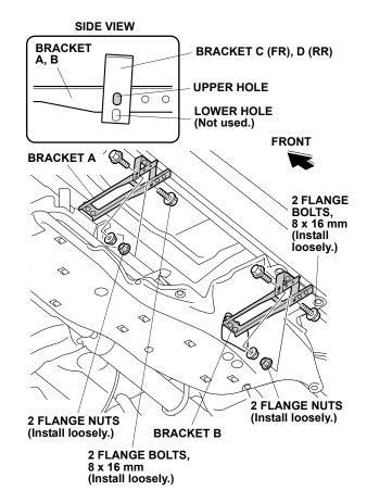
19. Secure the left running board to bracket A and bracket B with eight loosely-installed 8 x 16 mm flange bolts.
