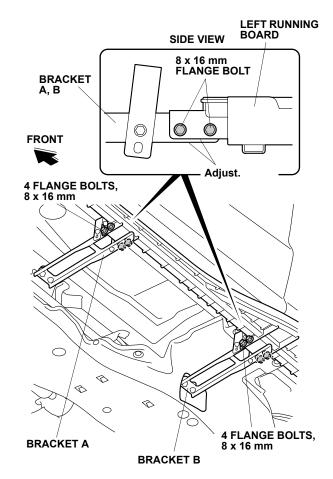
Adjust the position of the running board as shown. Tighten the four 8 x 16 mm flange bolts and four flange nuts loosely installed in step 18 in the order
