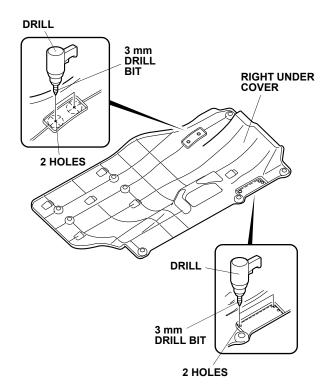
11. Enlarge two holes made in the right under cover in step 10 with a 10 mm drill bit.
