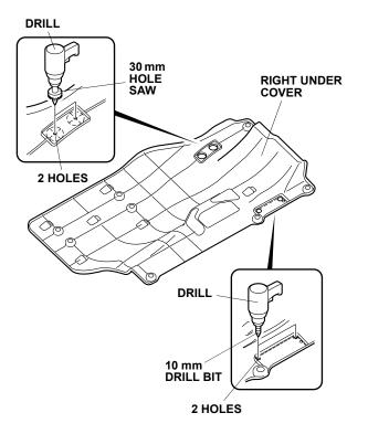
12. Enlarge two holes made in the right under cover in step 10 with a 30 mm hole saw. Remove any burrs.
