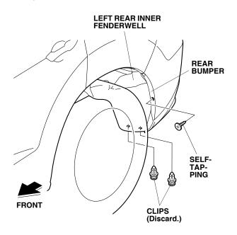
7. Remove and discard the two clips from the left rear inner fenderwell.
