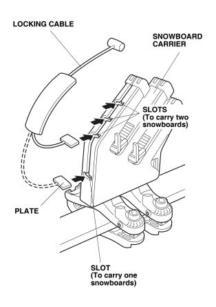
15. After loading the snowboards on the carrier, adjust them with the help of the board supports so that the top edges are level and the boards are as far down in the carrier as possible. To secure the snowboards, use the key to open the covers, and insert the locking cable stops into the holes in the carrier covers.
