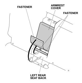
6. Secure the fastener to the bottom of the left rear seat back.
