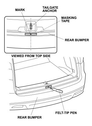
2. Align the rear bumper applique to the rear bumper and check the rear bumper applique installation position.
