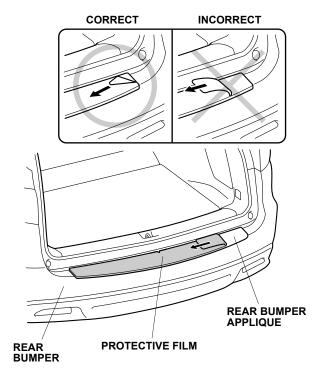
13. Repeat step 10 at the center of the lower section of the rear bumper applique.
