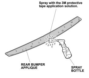
8. Align the v-notch on the rear bumper applique to the mark on the masking tape, and align the edge along the crease of the curved surface as shown. Smooth the rear bumper applique along the rear bumper.
