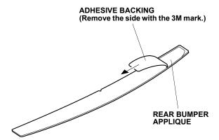
7. Spray the rear bumper applique with the 3M protective tape application solution.
