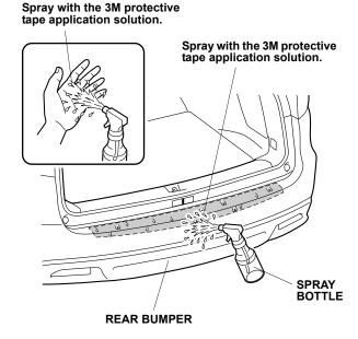
6. Remove the adhesive backing from the side of the rear bumper applique with the 3M mark.
