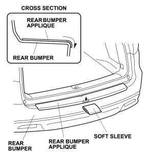
14. Repeat step 11 to smooth the left and right sides of the lower section of the rear bumper applique.
