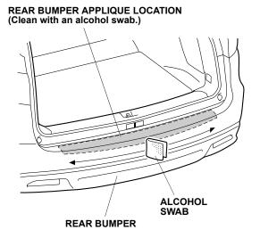
5. Using a spray bottle with the 3M protective tape application solution, spray the area where the rear bumper applique will attach. Spray some solution on your hands.
