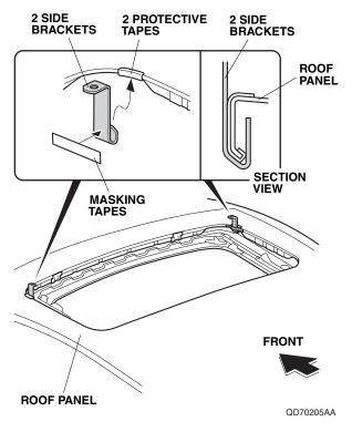
11. Repeat the same procedure to install the side bracket on the left side of the moonroof opening.
