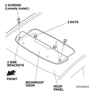
Position the moonroof visor with equal spacing on each sides. Check that the rubber molding is not twisted or rolled under the visor.
