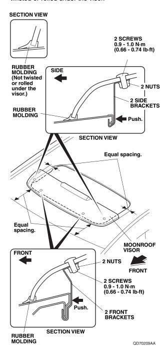
17. Tighten two screws and two nuts on each side of the vehicle first, then tighten two screws and two nuts on the front. Tighten while applying pressure so that there is no gap between the brackets and the roof panel. Torque the screws to 0.9 - 1.0 N·m (0.66 - 0.74 lb·ft).
