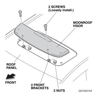
15. Loosely install the moonroof visor to the side brackets with two screws and two nuts. Remove the masking tapes from the side brackets.
