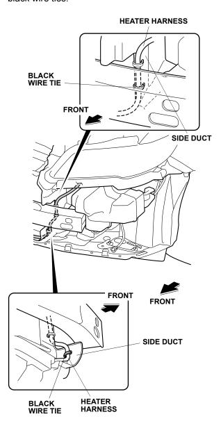
26. Secure the heater harness to the vehicle harness with one wire tie.
