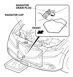
After the coolant drains, reinstall the radiator cap to prevent dirt and contamination from entering the radiator. 5. Apply masking tape to the front bumper, left headlight and left front fender as shown.
