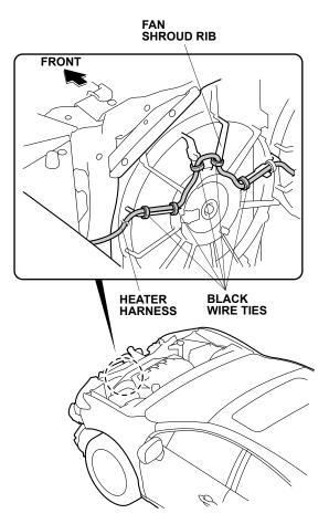
29. With the help of an assistant, route the heater harness through the front bumper opening, and reinstall the front bumper.
