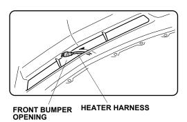
30. Install the protective cap to the front bumper as shown.
