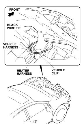
28. Secure the heater harness to the fan shroud ribs with five black wire ties.
