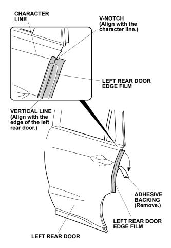
19. Align the vertical line on the left rear door edge film to the edge of the left rear door. While applying light pressure, carefully remove the adhesive backing.
