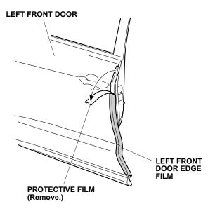
14. Starting from the center and working outward, use your finger and the soft sleeve to fold the left front door edge film inside the left front door as shown. Move the soft sleeve in one direction only. Do not damage the door seam sealant.
