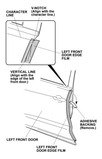
10. Align the vertical line on the left front door edge film to the edge of the left front door. While applying light pressure, carefully remove the adhesive backing.
