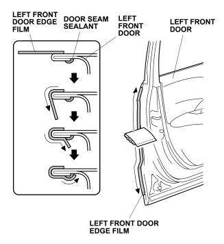
15. Using a shop towel, wipe the excess 3M protective tape application solution from the left front door edge film. Allow the left front door edge film to dry thoroughly.
