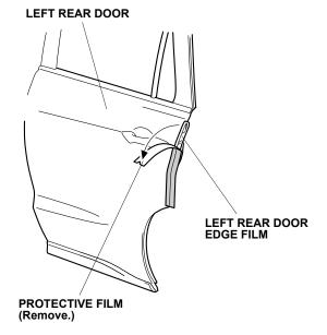
22. Starting from the center and working outward, use your finger and the soft sleeve to fold the left rear door edge film inside the left rear door as shown. Move the soft sleeve in one direction only. Do not damage the door seam sealant.
