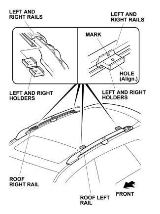
4. Align the hole in each holder with the mark on the inside of the roof rail.
