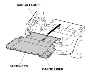
3. Secure the cargo liner to the left rear side trim with the fasteners.
