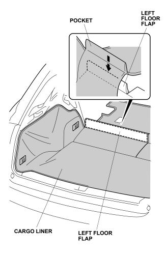
Secure the cargo liner to the left rear seat back with the fasteners. If the vehicle is equipped with a rear seat cover, release one fastener, fasten the cargo liner to the seat-back, then secure the seat cover to the cargo liner.
