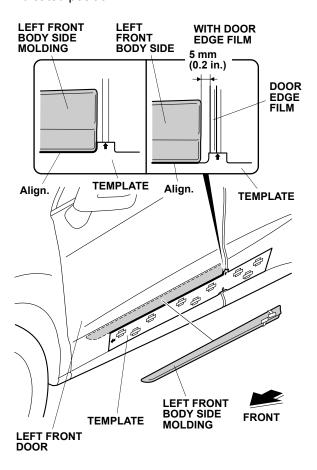
While applying light pressure against the left front body side molding, carefully remove the taped adhesive backings.
