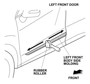
Peel back the adhesive backing from three adhesive strips, and tape the ends to the front surface of the body side molding. Remove the small pieces of adhesive backing.
