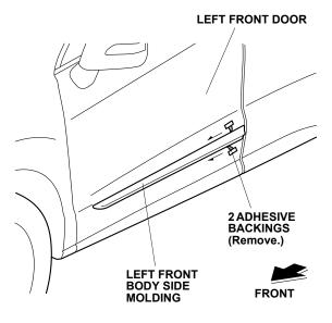
8. Using a rubber roller, apply pressure against the left front body side molding and roll from one end to the other.
