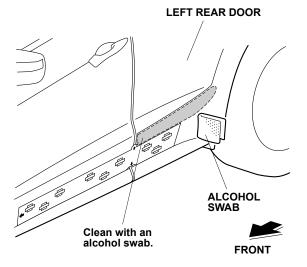
Peel back the adhesive backing from two adhesive strips, and tape the ends to the front surface of the body side molding with masking tapes. Remove the small pieces of adhesive backings.
