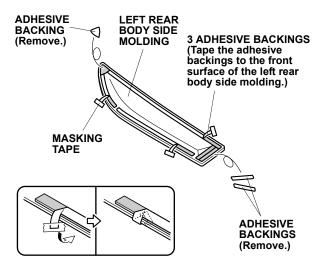
10. Align the left rear body side molding with the template and attach it to the left rear door as shown.
