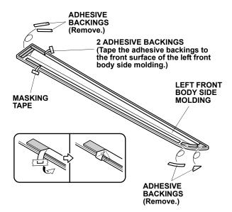
6. Align the left front body side molding with the template and attach it to the left front door as shown. NOTE: If the vehicle is equipped with door edge film, attach the left front body side molding at the indicated position.
