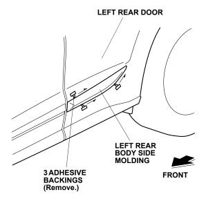
12. Using a rubber roller, apply pressure against the left rear body side molding and roll from one end to the other.
