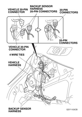
23. Secure the backup sensor harness to the vehicle harness with four wire ties.
