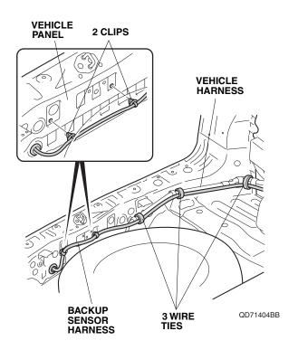
37. Secure the backup sensor harness to the vehicle panel with two clips on the backup sensor harness.
