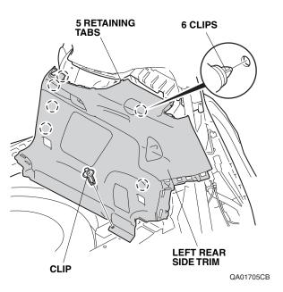
14. Release the wire and remove the lever, then remove the left rear side trim panel.
