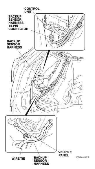
33. Secure the backup sensor harness to the vehicle panel and vehicle harness with one wire tie.
