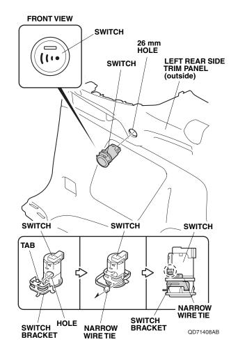
41. Align the tab on the switch bracket with the hole on the switch and secure the switch bracket to the switch with one narrow wire tie. NOTE: Firmly press the switch bracket against the left rear side trim panel, and make sure that there is no clearance between the switch and left rear side trim panel. 42. Remove and discard the vehicle clip.
