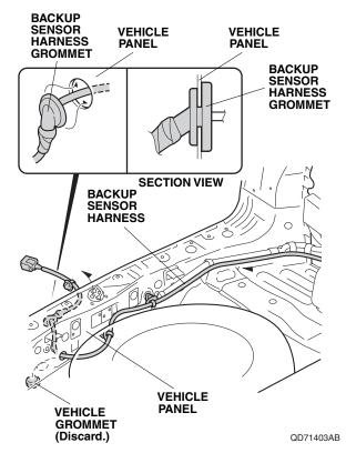
35. Route the backup sensor harness through the hole, and seat the grommet on the backup sensor harness in the vehicle panel hole.
