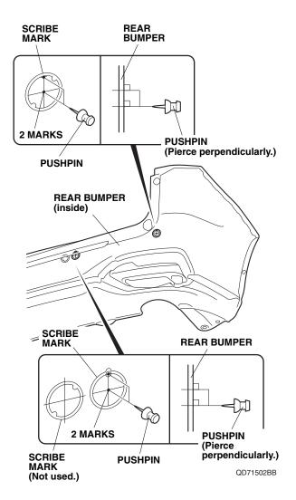
48. While wearing eye protection, drill the eight pierced marks with a 3 mm drill bit from the painted side of the rear bumper.
