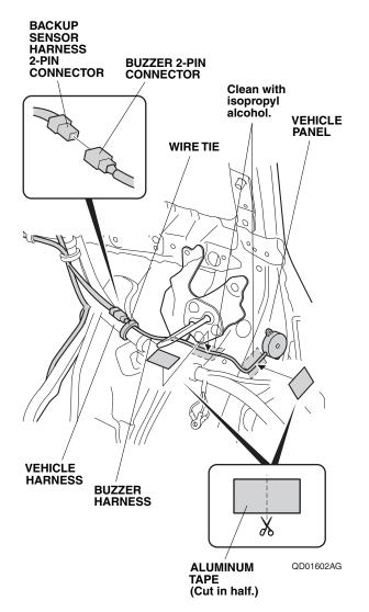
28. Plug the backup sensor harness 2-pin connector into the buzzer 2-pin connector.
