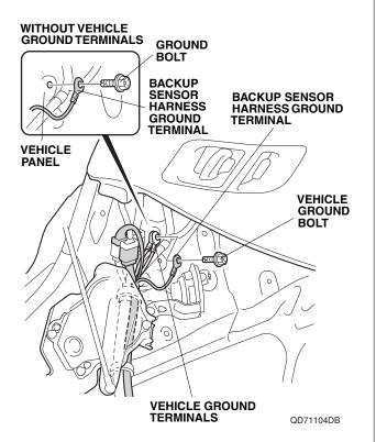
25. Secure the backup sensor harness ground terminal to the vehicle ground terminals with the vehicle ground bolt just removed. Do not put the ground terminal calkings on top of one another. 26. Using isopropyl alcohol on a shop towel, thoroughly clean the vehicle panel where the buzzer will attach.
