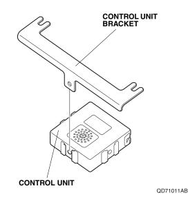
20. Loosen the two vehicle bolts from the vehicle panel, and install the control unit bracket between the vehicle panel and vehicle unit bracket with the two vehicle bolts just loosened.
