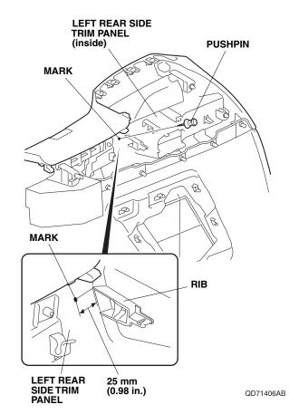
39. While wearing eye protection, drill the pierced mark on the left rear side trim panel with a 3 mm drill bit. Then enlarge the 3 mm hole to 26 mm using a 26 mm hole saw.
