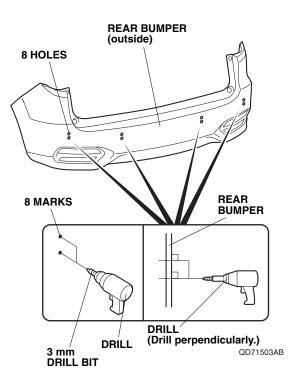
49. While wearing eye protection and drilling from painted side of the rear bumper, enlarge the two lower 3 mm outer holes to 24 mm using a 24 mm hole saw.
