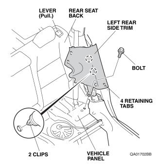
8. Pull the lever, and fold down the rear seat back.
