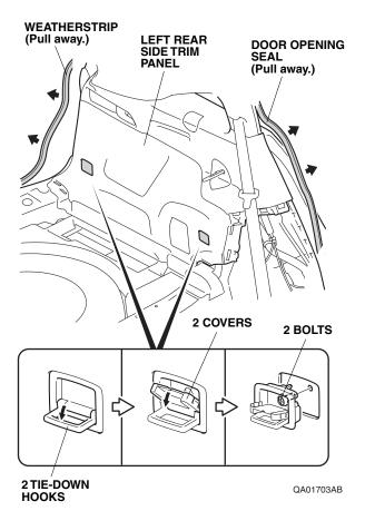
10. Using an impact screwdriver, remove the two tiedown hooks. 11. Gently pull the lever on the left rear side trim panel, and use a small flat-tip screwdriver wrapped with a shop towel, remove the inner handle cap.
