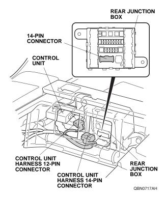
24. Plug the control unit harness 12-pin connector into the control unit.
