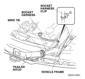
32. Secure the socket harness to the trailer hitch with one wire tie.
