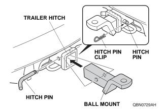
After the first 600 miles (1,000 km) of towing, have your Acura Dealer check the tightness of the trailer hitch bolts.
