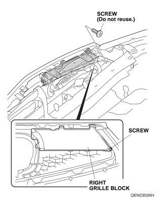
Using diagonal cutters, cut the top right corner • tab to pull out the right grille block.
