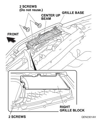
Using a ratchet, T20 TORX bit, and 2 in. long 1/4 in. drive extension bar, remove two screws.
