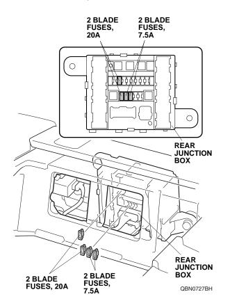
38. Using isopropyl alcohol on a shop towel, thoroughly clean the rear junction box cover where the fuse labels will attach.
