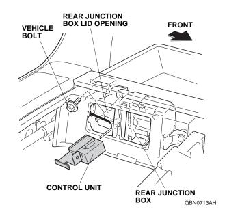
20. Position the control unit bracket as shown, and secure the control unit bracket with the vehicle bolt.
