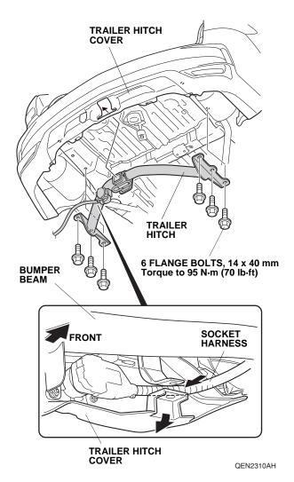
14. Torque the six 14 x 40 mm flange bolts to 95 N·m (70 lb·ft).
