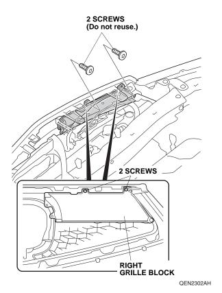
Using a ratchet and T20 TORX bit, remove one screw.
