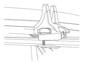
6. Slide the latch on one attachment strap into the clip on a base.
