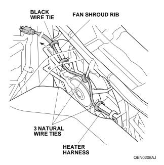
17. Route the heater harness through the front bulkhead and secure the heater harness to the vehicle harness with three black wire ties.
