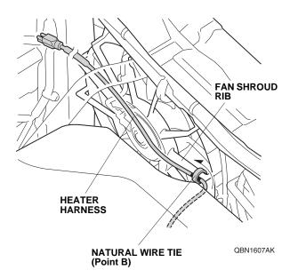
16. Route the heater harness across the fan shroud and secure the heater harness to the fan shroud ribs with three natural wire ties and one black wire tie.
