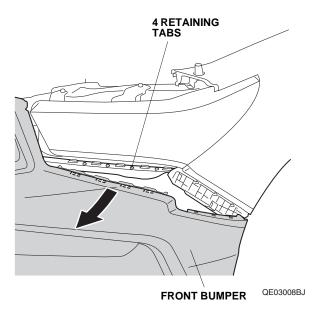
• With the help of an assistant, release the front bumper and unplug the vehicle connectors.
