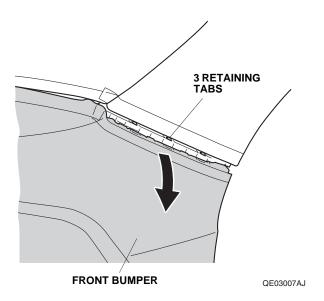
With the help of an assistant, release the four retaining tabs on each side.
