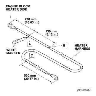
9. Install the one wire tie with clip to the heater harness at point  $\boxed{A}$  as shown.
