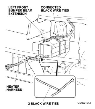
21. With the help of an assistant, route the heater harness through the front bumper center lower grille, then install the front bumper.
