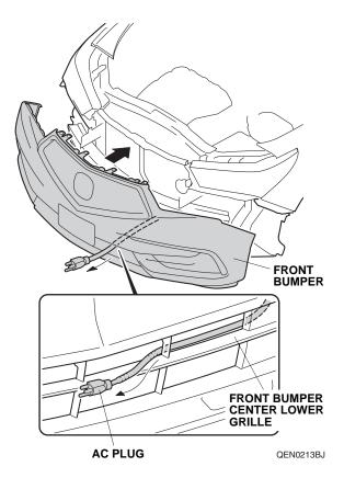
22. Secure the heater harness to the front bumper center lower grille with two black wire ties.
