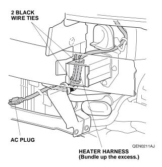
20. Connect two black wire ties together and secure the heater harness to the left front bumper beam extension with the connected black wire ties.
