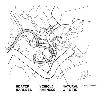
15. Route the heater harness toward the fan shroud and secure the heater harness to the fan shroud rib with the one natural wire tie at the point B.
