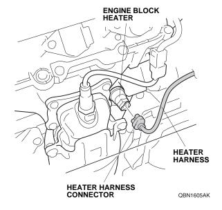
13. Route the heater harness in the direction shown and secure the heater harness to the vehicle bracket with one wire tie with clip installed in step 9.
