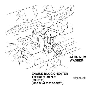
12. Plug the heater harness connector into the engine block heater.
