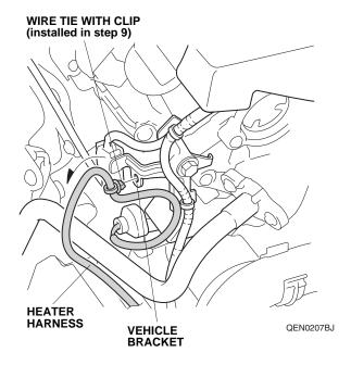
14. Secure the heater harness to the vehicle harness with one natural wire tie.
