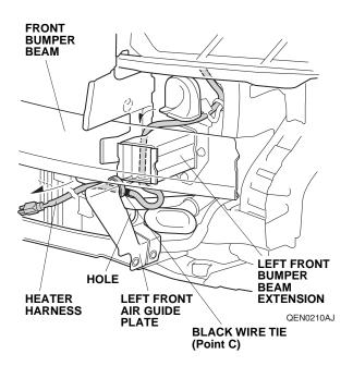
19. Line up the AC plug with the middle of the vehicle. If you have excess heater harness, bundle it up and secure it with two black wire ties as shown.
