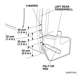
6. Using a utility knife, remove the undercoating in the areas shown.
