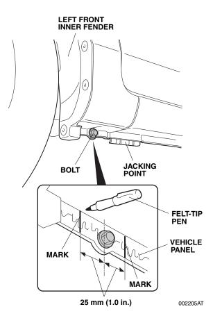
2. Remove the bolt from the bottom of the left front fender.
