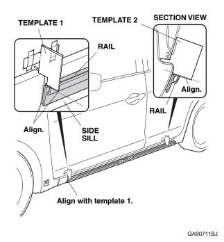
20. While holding the rail in place, slowly and carefully remove each adhesive backing.
