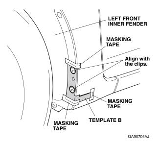
10. Using a felt-tip pen, mark the left front fender as shown.
